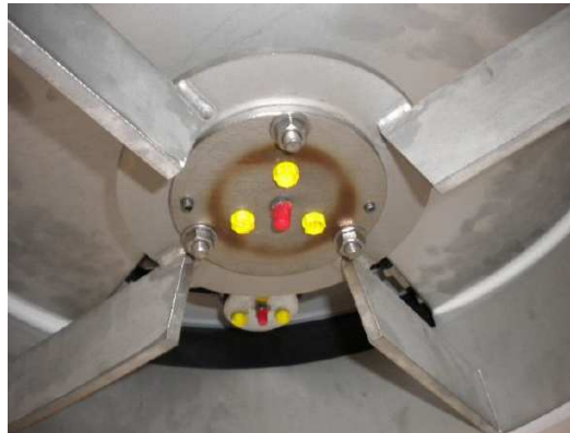
new stainless steel housing bearing arrangement
